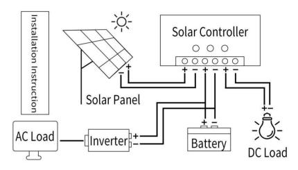
When connecting the controller, be sure to connect the battery first, then the solar panel.
